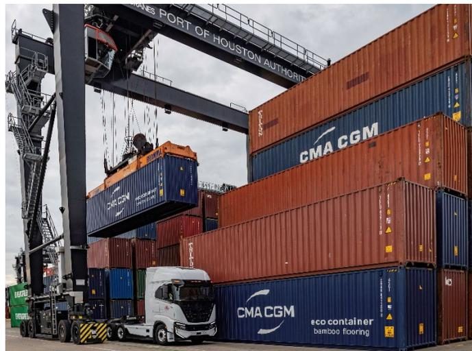
*Zero-emissions drayage truck receiving a container at Bayport Container Terminal*
