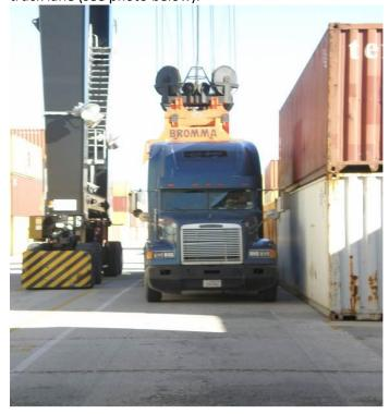
5.5.3. Trucks must be properly aligned in the truck lane for RTGs to safely land and hoist containers to and from chassis. (See photo below shows how a truck should **NOT** be in the RTG pad).
