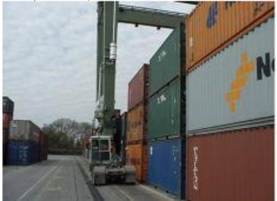
5.5.12. When traveling, the RTG operator cannot see all 16 wheels of the RTG. In this photo, the operator cannot see the truck parked on the south crane runway of the RTG Pad.
