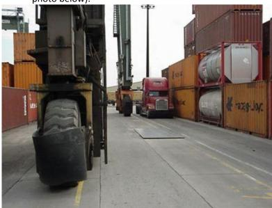
5.5.8. The RTG operator may sound a horn to assist a truck driver in correctly positioning the truck and chassis under the RTG. The horn is sounded once to signal the truck driver to pull forward. The
