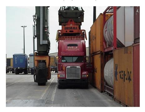
5.5.3. Trucks must be properly aligned in the truck lane for RTGs to safely land and hoist containers to and from chassis. (See photo below shows how a truck should **NOT** be in the RTG pad).
