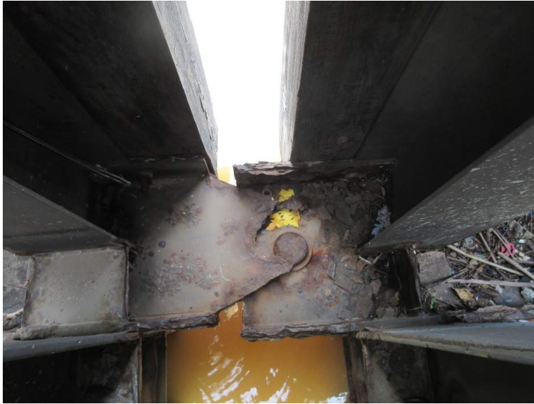
Figure 6. Failed pin connection at joint in secondary framing at Bent 1.
