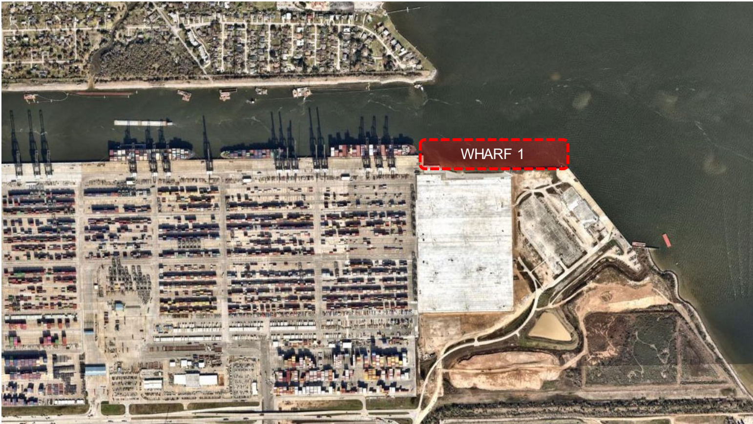
Construction of approximately 1,600 feet of new wharf structure at the Bayport Container Terminal. The project scope includes surveying, dredging, drilled shaft foundations, structural concrete, crane rails, fender systems, utilities, and a stevedore support building.
