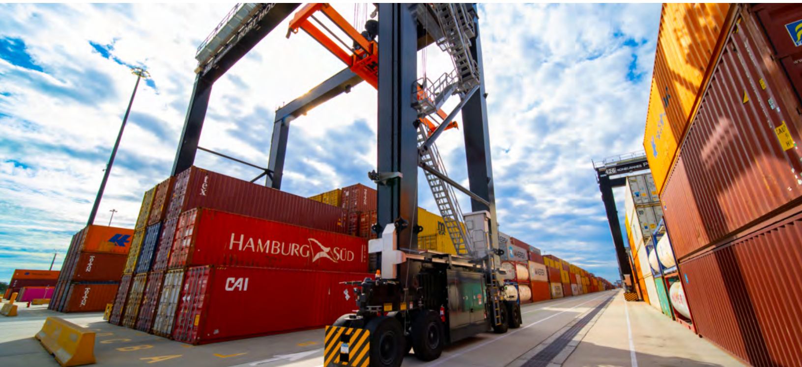
Figure 5.3: Photo of RTG Crane
